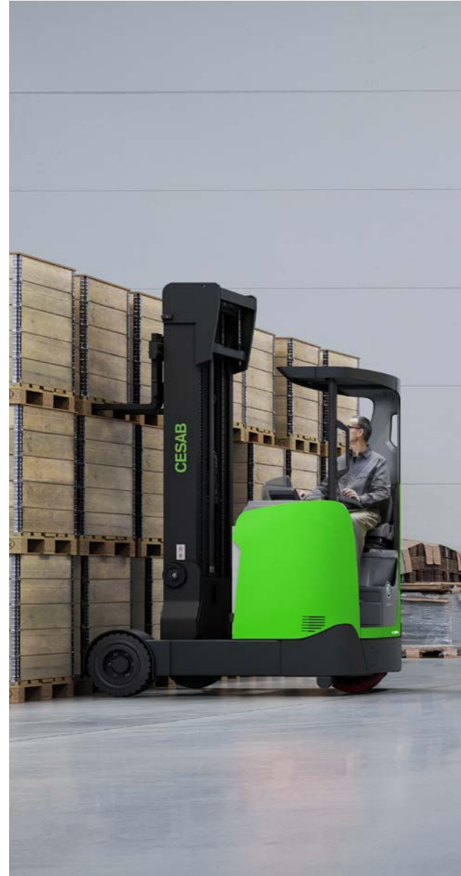
The CESAB R300 Outdoor can handle road gradient and transition lines thanks to soft and elastic tyres, a durable drive wheel made from Redthane, and 145 mm ground clearance.
