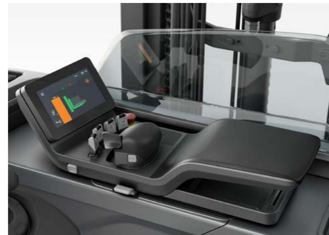
The adjustable mini-joystick console allows for accurate fingertip control.
