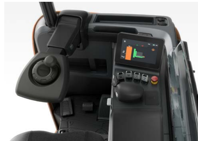
The operator compartment offers many different storage as well as dedicated space for PC with power outlet and a USB connector.
