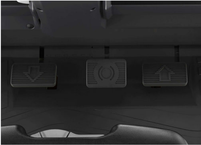
Different pedal layouts are available to fit drivers' preferences. Double accelerator pedals allow the operator to change driving direction with the feet.
